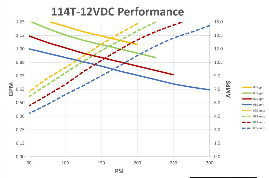
Data recorded pumping water at room temperature and fully charged battery at 13VDC. Performance will vary with voltage fluxuations, application, and mfg tolerances. Copyright Pumptec Inc. 2020
