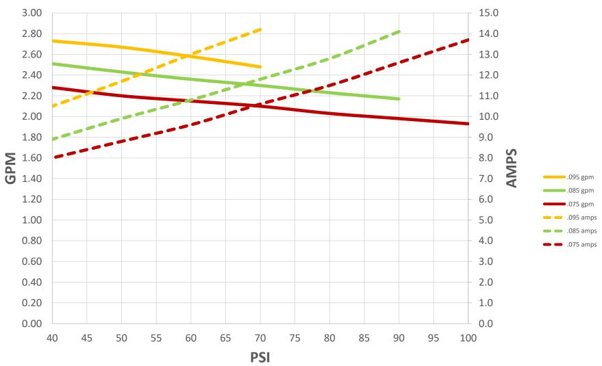
Data recorded pumping water at room temperature and fully charged battery at 13VDC. Performance will vary with voltage fluxuations, application, and mfg tolerances. Copyright Pumptec Inc. 2020
