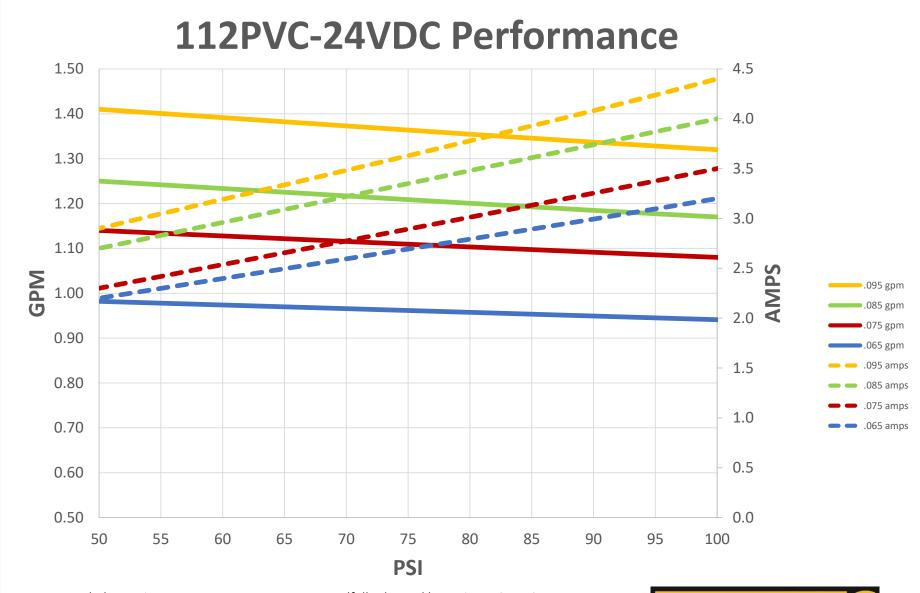
Data recorded pumping water at room temperature andfully charged batteries at 24VDC. Performance will vary with voltage fluxuations, application, and mfg tolerances. Copyright Pumptec Inc. 2020
