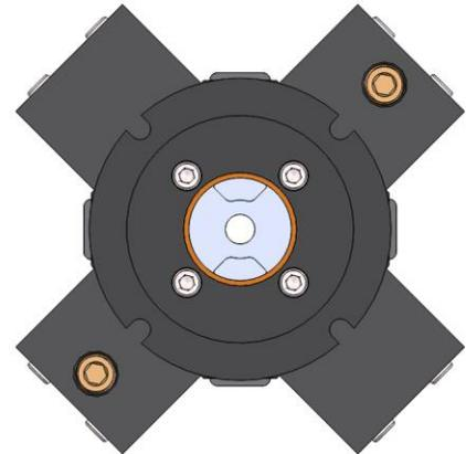
18. Slide pump onto motor and tighten flange head bolts.
