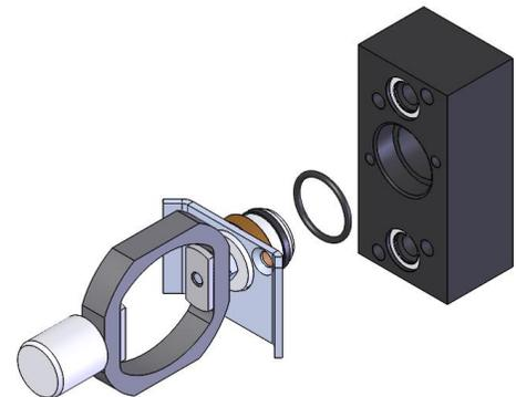
7. Tighten bolts to secure retainer plate. Remove hoop plunger. Replace valve washers if needed. A small amount of grease helps keep the washers in the pockets. Repeat steps 5, 6, and 7 for other three heads.
