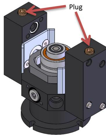
12. Flip other hoop assembly so plugs are down. Slide hoop onto driveshaft. Start bottom bolts on heads.
