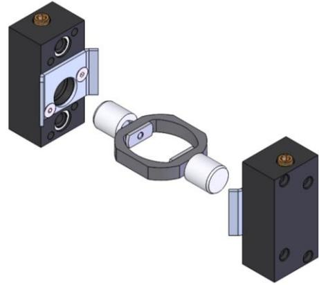
11. Slide hoop plunger/head assembly onto driveshaft with the plugs facing up. Start bottom bolts on heads.
