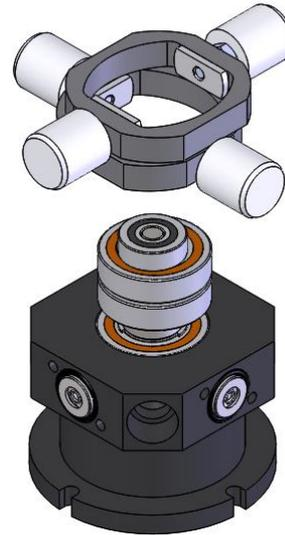
5. Remove bolts and then retaining plate from head. Remove guide, seal ring, and O-ring from head.
