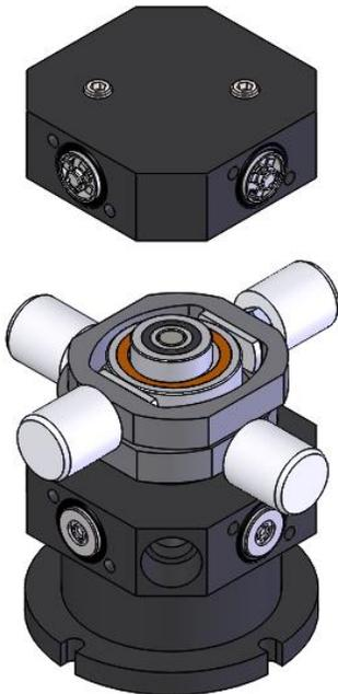
4. The hoop plungers can also be removed. Clean parts that are being reused.
