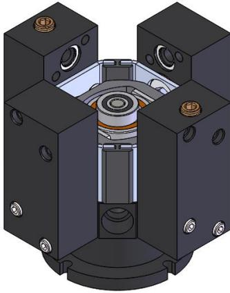
14. Pull heads apart slightly. Note orientation of inlet is opposite of outlet before sliding manifold into place. Slide inlet manifold with bearing housing onto top of driveshaft.
