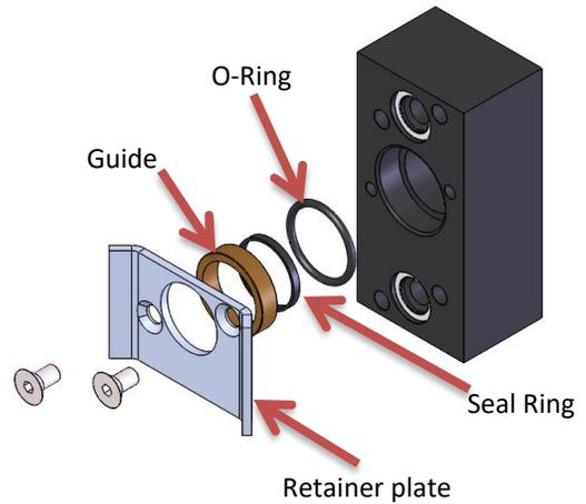
6. Grease seal ring and O-ring. Place O-ring into head. Slide retainer plate, guide, and then seal ring onto the plunger and install into head.
