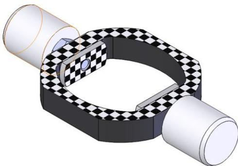
10. Place one head onto each end of plunger hoop. Do this for both hoop plungers.
