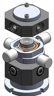
4. The hoop plungers can also be removed. Clean parts that are being reused.
