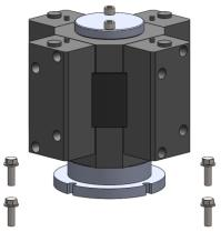
2. Separate heads from pump. Remove rubber protectors. Repeat step for other three heads.
