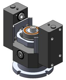
15. Slide hoop plunger and "Head B" assembly onto driveshaft. Start bottom bolts on heads.
