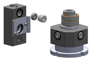
11. Apply grease to checkered areas of both hoop plungers.
