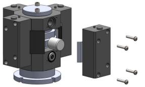
3. The inlet manifold can now be removed by lifting them off the driveshaft.
