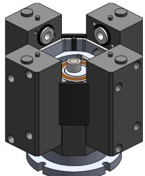
17. Pull heads apart slightly. Note orientation of inlet is opposite of outlet before sliding manifold into place. Slide inlet manifold with bearing housing onto top of driveshaft. Push heads together onto manifolds. Manifold should slide easily and completely over valves.
