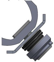
10. Replace valves and o-rings in outlet manifold. Replace o-rings and inserts into inlet side of heads. Note valve orientation. A little bit of grease on the o-ring will make the valves stay in the pockets.
