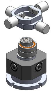
5. Remove bolts and then retaining plate from head. Remove guide, seal ring, and o-ring from head.
