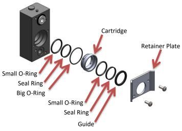
6. Grease seal ring and o-ring. Place big and small o-rings into head.
