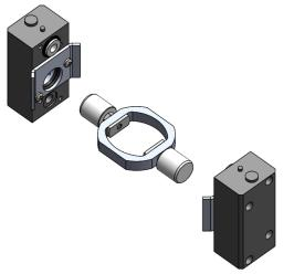
14. Slide hoop plunger and "Head A" assembly onto driveshaft. Start bottom bolts on heads.
