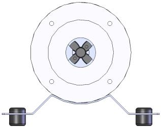
20. Orient coupling in pump so jaws are vertical.
