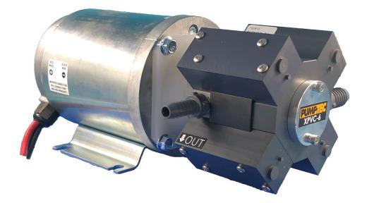
The Pumptec XPVC high flow pump features solid ceramic 4 plunger design and dual PTFE seals. You can count on having the pressure and high flow you need for the most demanding Soft Wash jobs. Like all Pumptec pumps, you can look forward to a long and problem-free life. The XPVC features a machined PVC body and alloy C-276 valves for maximum chemical compatibility.
