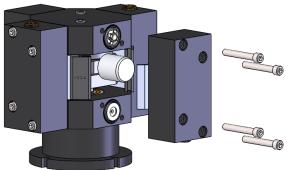
3. The inlet manifold can now be removed by lifting them off of the driveshaft.
