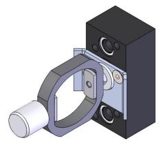
8. Replace valves and O-rings in both outlet and inlet manifolds. Note valve orientation. A little bit of grease on the O-ring will make the valves stay in the pockets.
