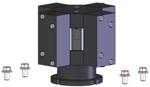
2. Separate heads from pump. Rubber protectors can also be removed. Repeat step for other 3 heads.
