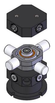
4. The hoop plungers can also be removed. Clean parts that are being reused.
