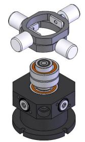
5. Remove bolts and then retaining plate from head. Remove guide, seal ring, and O-ring from head.
