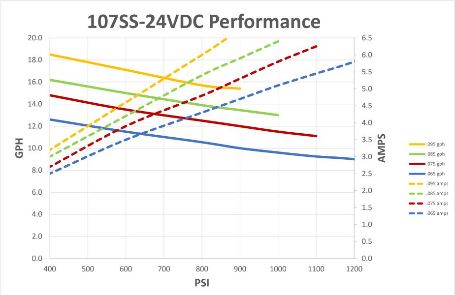
Data recorded pumping water at room temperature and fully charged battery at 24VDC. Performance will vary with voltage fluxuations, application, and mfg tolerances. Copyright Pumptec Inc. 2020
